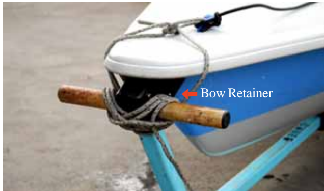
5. Place the bow of the boat onto the curved plastic bow retainer, and then secure the boat using the painter with a series of half hitches. Please see intermediate knot section of the manual for instructions on how to tie a half hitch.
