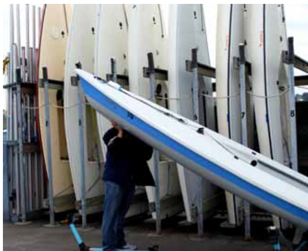
5. Place the bow of the boat onto the curved plastic bow retainer, and then secure the boat using the painter with a series of half hitches. Please see intermediate knot section of the manual for instructions on how to tie a half hitch.
