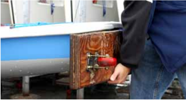
20. Make sure the wheels of the stern dolly are in the correct slot to return the boat. Untie the painter and lift the bow up. The stern dolly should catch the ground and be secure. Gently lift the boat until it is almost vertical, and then begin sliding it into the appropriately numbered slot.
