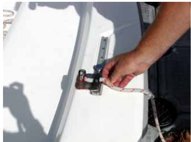
22. Provided that the tide is not extremely low you may put on the rudder . Pass the rudder under the traveler (the bridle which controls the sideways movement of the boom). If the tide is low you will put the rudder on after the boat is brought to the windward side of the dock.
