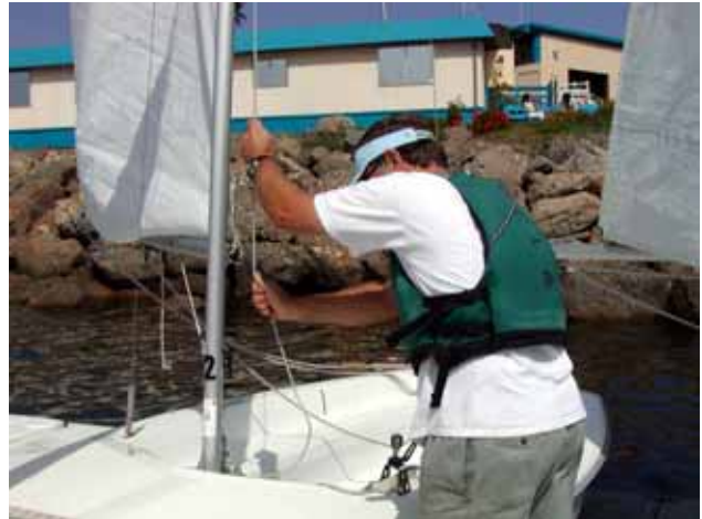
21. Lead the jib sheets through the fairleads OUTSIDE the shrouds, and secure them by tying a figure eight stopper knot close to the end of each sheet (refer to page 28). NB: At least six inches of line should be free at the bitter end (extreme end of a line).
