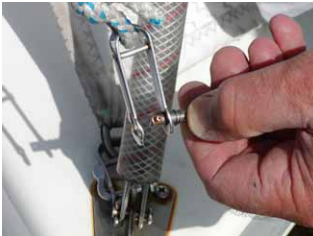
18. Attach the jib halyard to the head of the jib using the jib shackle.
