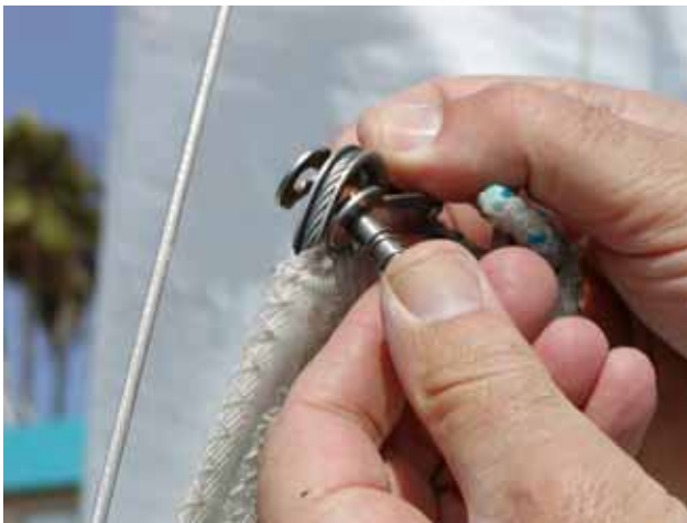
19. Attach the hanks on the jib luff to the forestay.
