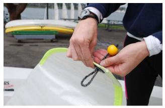
8. Take the ball at the end of the main halyard and pull it over the top of the sail towards the loop that was passed through the grommet of the head of the mainsail. Put the ball into the loop and pull taut.
