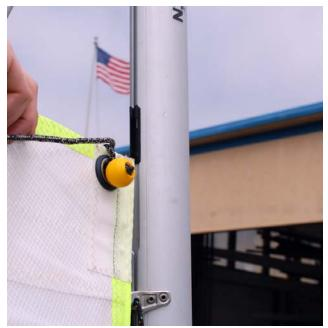
10. Raise the mainsail using the main halyard which is on the starboard side of the mast until the mast reaches the top of the mast. The crew should use their hand to guide the boltrope as the skipper raises the sail.
