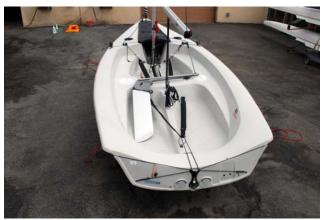
2. Insert the drain plug, into the transom and seal the hull by turning the plug clockwise.
