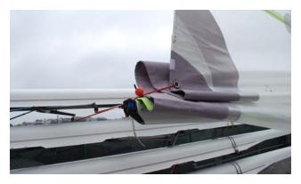
19. Provided that the tide is not extremely low you may attach the rudder by placing the pintles into the gudgeons. Please note that the bungee cord for the hiking strap should be under the top gudgeon.
