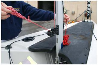
4. Uncleat the main halyard from the starboard side of the mast.
