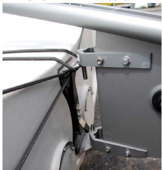
20. Uncleat the jib furling line. It is located on the starboard side of the cockpit.
