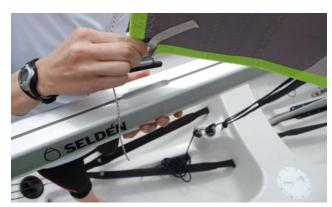
12. Attach the outhaul of the sail (located on the port side of the boom) using the same ball and loop method used for the main halyard.
