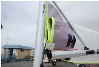
18c.Slab reef the aft portion of the mainsail while lowering the mainsail. Recleat the main halyard.
