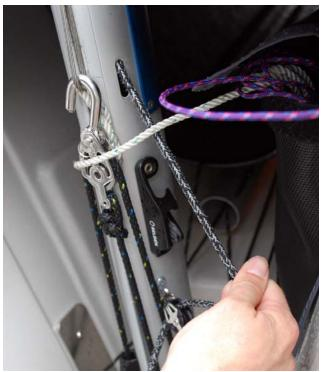
5. Release the main halyard slowly so that the boom will be lowered gently into the cockpit of the vessel.
