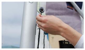
17. Pass the cunningham through the clam cleat on the port side of the mast and tie a bowline into the end of the line.
