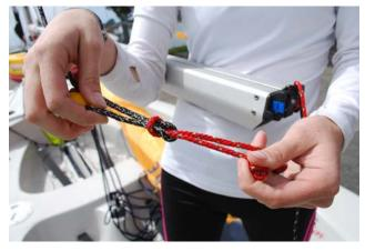
12. Sheet-in on the mainsheet until it is taut. Then place the coiled mainsheet on to the maincleat.
