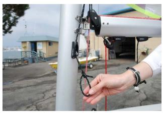
18a.**OPTIONAL REEFING STEPS**: Remove the Cunningham from the cleat and grommet. Pass it through the reefing grommet on the port side which is directly above the cunningham grommet.
