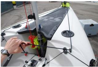
20. Push the boat off the floating dock and walk it to the windwardside of the dock. Then drop the centerboard by pulling on the centerboard handle.
