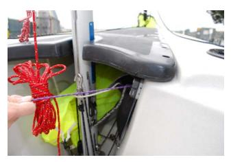
19. Sheet in on the starboard jib sheet to unfurl the jib. Make sure the Spinnaker halyard does not catch the sail as it unfurls.
