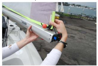
13a.**OPTIONAL REEFING STEPS**: Take the reefing line on the starboard side of the boom and pass it through the top reefing crigle from the port side. Then thread the line through the second cringle on the starboard side. Then thread the line through the bottom cringle on the port side.
