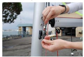
7. Uncleat the main halyard and slowly begin lowering the sail. The sail should be ROLLED as it is lowered as it is made of mylar and should never be crumpled up for transport. Be sure to roll the mainsail so that the leech is flush.
