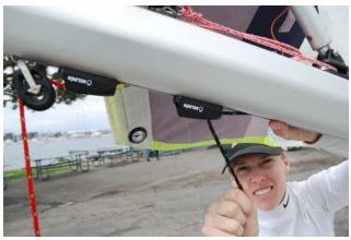
5. Untie the ball and loop used for the clew. Then lower the boom to the cockpit.
